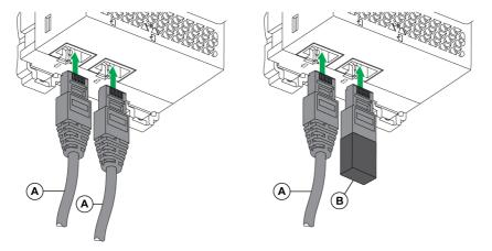
A Circuit breaker BCM ULP cord or RJ45 male/male ULP cord B ULP line termination
