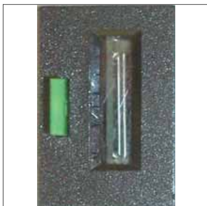
J Normal indicator view (no fault).
