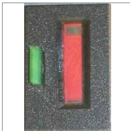
J Indicator showing a fault (red).
