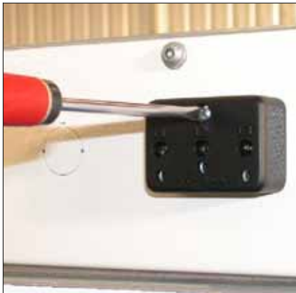
J Unscrew the two side screws (flat headed screwdriver).
