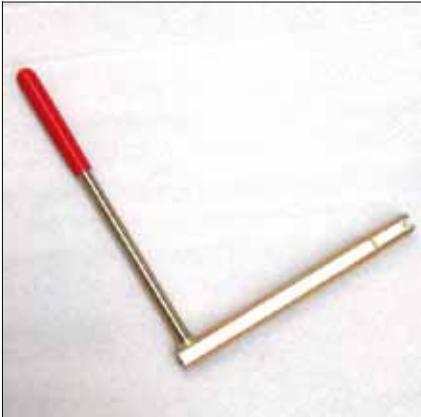
J Standard operating lever for the earthing switch (red end).
