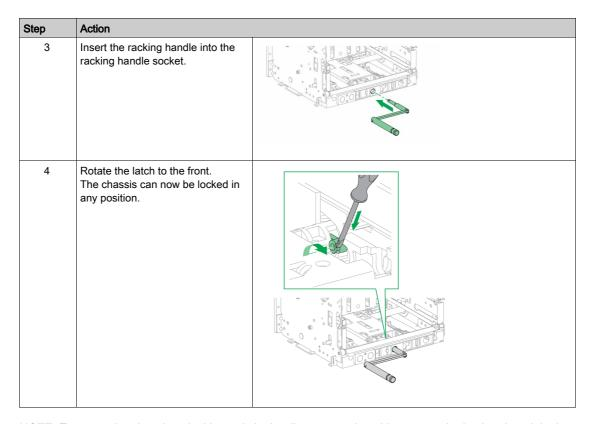
**NOTE:** To return the chassis to locking only in the disconnected position, rotate the latch to its original position at the rear.
