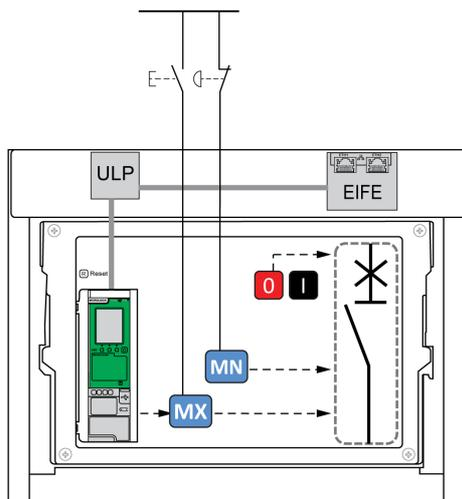
The open orders on MN or MX voltage releases by external pushbutton can be maintained to force the circuit breaker in open position and reject any close order. The Micrologic X open orders are not maintained.
