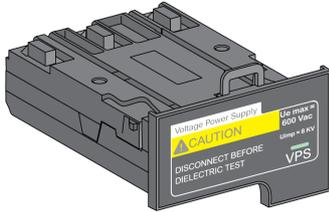
The VPS module is installed in the lower part of the Micrologic X control unit and can be replaced. A green LED on the front face indicates that the VPS module is powered and a 24 Vdc output is supplied. For information on spare part replacement and installation, consult the instruction sheet on the Schneider Electric website: [NVE40741](http://www.se.com/nve40741)
