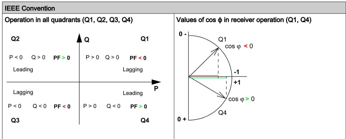
**NOTE:** For a device, a part of an installation which is only a receiver (or generator), the advantage of the IEEE convention is that it adds the type of reactive component to the PF and cos φ indicators:
