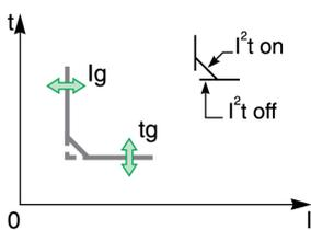
The ground-fault protection threshold I<sub>g</sub> sets the level of ground-fault current at which the circuit breaker trips when reaching the ground-fault protection time delay t<sub>g</sub>.
