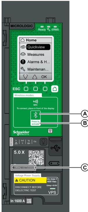
Using Bluetooth low energy BLE communications, you can access the Micrologic X control unit from a smartphone running the Masterpact MTZ Mobile App (see page 16). This application offers a task-oriented interface with the control unit. You can establish a BLE connection with only one Micrologic X control unit at the same time. Only one smartphone at a time can connect to a control unit.
