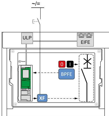
**NOTE:** The BPFE electrical closing pushbutton can be connected to Micrologic X control unit, as shown in the preceding diagram. In this case the control unit manages the closing function and the closing orders from the BPFE. The BPFE closing order is available in both Manual and Auto control modes.
