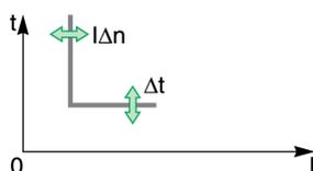
Earth-leakage protection is definite time.
