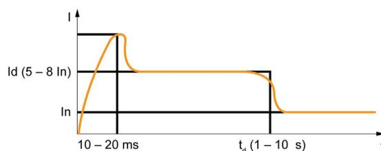
**NOTE:** Masterpact MTZ1 L1 type circuit breakers are equipped with an additional fast instantaneous trip set at  $10 \times I_n$ .
