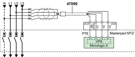
The VPS module can be supplied from an external voltage by means of the optional PTE voltage measurement inputs and voltage transformers (mandatory for voltages above 600 Vac).
