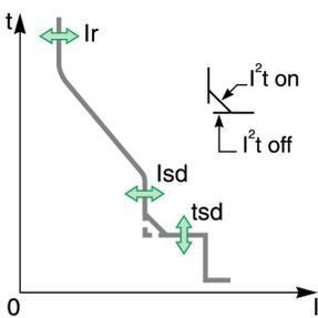
The short-time overcurrent threshold I<sub>s d</sub> sets the level of short-circuit current at which the circuit breaker trips when reaching the short-time overcurrent time delay.
