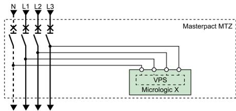
The input voltage of the VPS module is limited to 600 Vac. The module is directly connected to the internal pick up voltage (PTI) on the downstream side of the circuit breaker.
