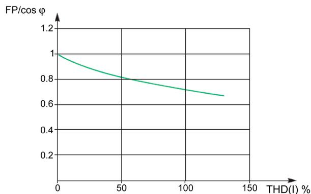
By comparing the 2 values, it is possible to estimate the level of harmonic deformation on the supply.
