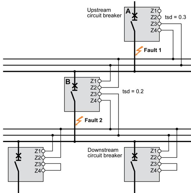
**NOTE:** On device **A**, the tsd and tg tripping delays must not be set to zero because this would make selectivity impossible.
