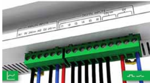
Power supply to analogue and digital inputs
