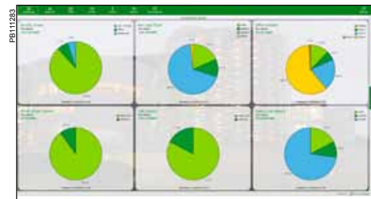
Consumption details by area and load type
