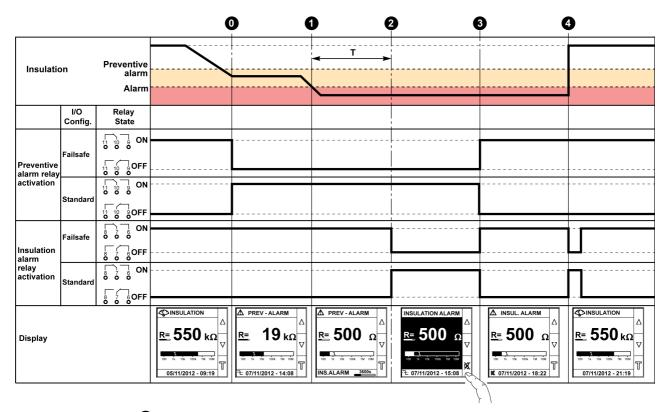
• After correcting the insulation fault in the power system, the insulation fault alarm relay toggles for 3 s.
