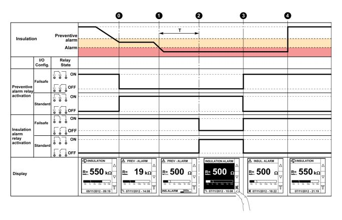
4 After correcting the insulation fault in the power system, the insulation fault alarm relay does not toggle for 3 s.
