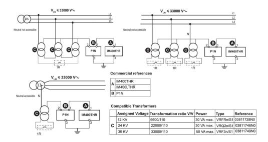
**NOTE:** Ensure that maximum voltage between pins 2 and 3 of P1N ground adaptor is less than 250 Vac, 400 Vdc.
