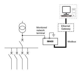
The Ethernet gateway can be an EGX series or Com'X series, for example.
