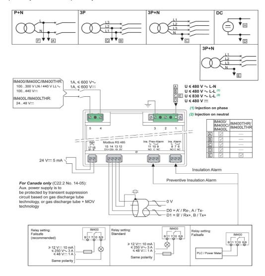
The relay operating mode (failsafe or standard) is controlled via the HMI of the Vigilohm device or with Modbus communication.
