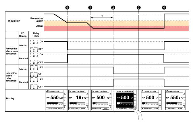
3 Insulation fault alarm acknowledgement does not switch back the relays to their initial position.
