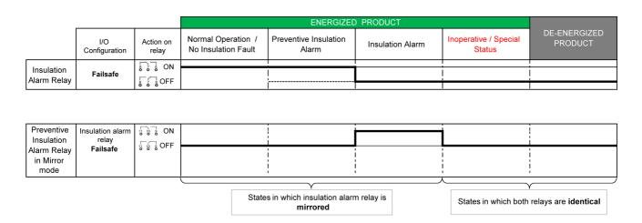
This allows you to easily separate an Insulation Fault signal from an Inoperative Product signal by implementing a series of simple wiring (or connection to a PLC).
